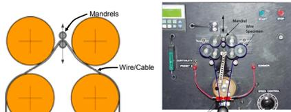
Cables are tested in cyclic fatigue via bending over a mandrel. Mandrel radius controls stress and strain experienced by electrodes/wires.
