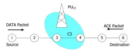
Fig. 1. PU occupies its licensed channel
