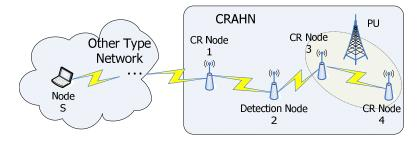
Fig. 4. End-to-end transmission
