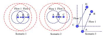
Fig. 5. Scenario 1 is for the comparison between SDMAC and DMAC; Scenario 2 is for the comparison between SDMAC and Circular-DMAC. In this two scenarios, Small circle stands for transmission range and big circle stands for the sensing range. Scenario 3 is for the comparison between SDMAC and DMAC-DA.
