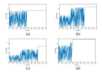
Fig. 5. Learning curves of the attacker and the system operator in the IEEE 118-bus system. (a) Attacker's strategy on line 9 at state 0. (b) System operator's strategy on line 7 at state 0. (c) Attacker's strategy on line 8 at state 9. (d) System operator's strategy on line 9 at state 9.
