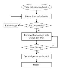
Fig. 1. Flow chart for the power system after being attack.
