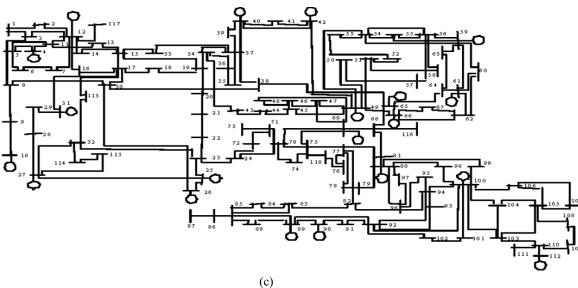
Fig. 2. IEEE standard bus systems. IEEE (a) 9-bus system, (b) 30-bus system, and (c) 118-bus system.
