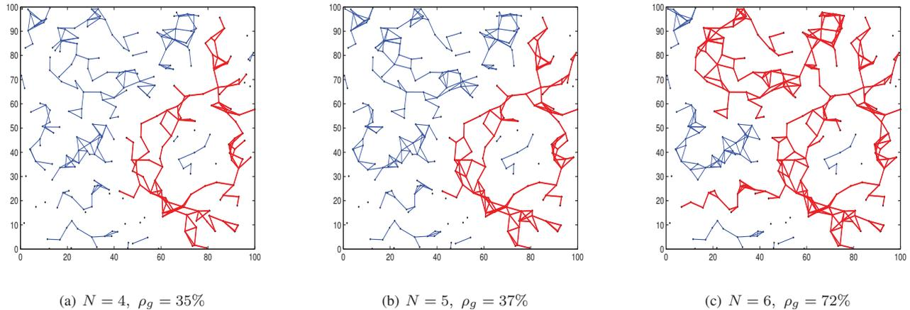
Fig. 9. An example of phase transition according to the number of channels  $N$  ( $\gamma_p = 0.2$ ,  $\mu_p = 0.4$ ). (When  $N$  grows from 4 to 5,  $\rho_g$  increases slightly (from 35% to 37%, shown in (a) and (b)). When  $N$  increases to 6, a giant component  $\rho_g = 72\%$  is formed (shown in (c)).)
