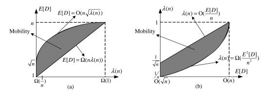
Fig. 4. Trade-offs among capacity, delay, and mobility. (a) An upper bound and a lower bound on the expected average packet delay when an achievable per-node throughput ranges from  $\frac{1}{n}$  to 1. (b) An upper bound and a lower bound on the per-node throughput when an upper bound on the expected average packet delay ranges from  $\sqrt{n}$  to n. We ignore the logarithmic terms in both cases as in [16].
