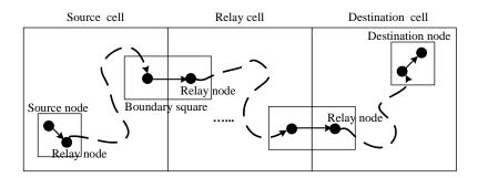
Fig. 3. An example for relaying a packet for a source-destination pair. The dotted lines mean that the relay nodes will carry a packet moving around until it hits a boundary square, or the square where the destination node lies.
