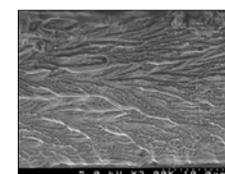
Fracture Surface of Ribbon Sample Tested in Tension  $\sigma_y = 1663$  MPa
