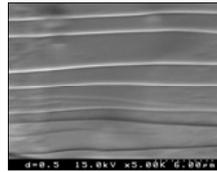
Shear Bands in Ribbon Bent over 0.50 mm mandrel
