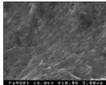
Fine Fatigue Striations in Ribbon Tested in Cyclic Fatigue Test Using Mandrel Diameter of 9.92 mm
