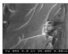
Fracture Surface of Ribbon Tested in Notch Toughness  $K_q = 96.4$  MPa m<sup>1/2</sup>
