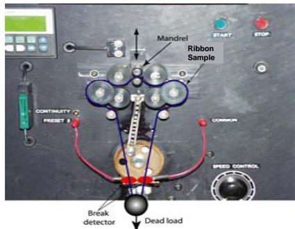
Flex tester used to conduct cyclic fatigue tests on the  $Fe_{78}Si_9B_{13}$  ribbon. Cyclic frequency = 1 Hz. Break detector automatically detects failure and stops cycle counter.
