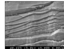
Shear Bands in Ribbon Bent over 0.225 mm mandrel
