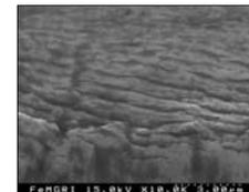
Coarse Fatigue Striations in Ribbon Tested in Cyclic Fatigue Test Using Mandrel Diameter of 1.19 mm
