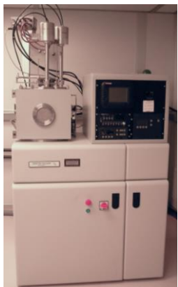
Denton Vacuum Sputtering System
