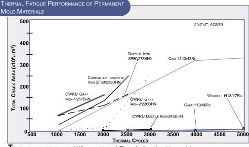
The best material above is H13 wrought steel. The selection of mold materials depends on the number of castings to be purchased since the cost of the steels is increased.
