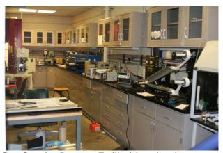
Case Capacitor Prototype Facility lab equipped to fabricate sealed nominally 100-F-size electrochemical capacitors from basic materials.
