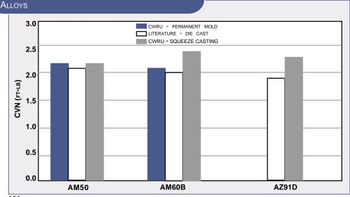
With the proper processing conditions, very good test bar results were obtained for permanent molds.
