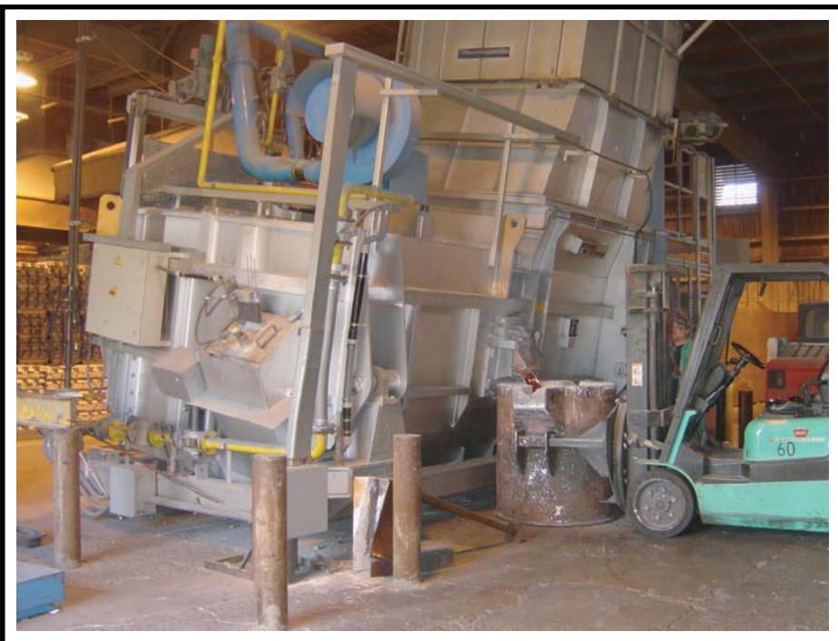
Tapping out molten aluminum from a tilting stack furnace
