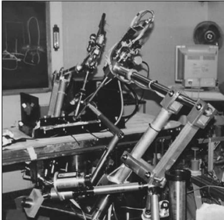
Figure 2.2: Second generation robotic telesurgical workstation from UCB and UCSF [1].
