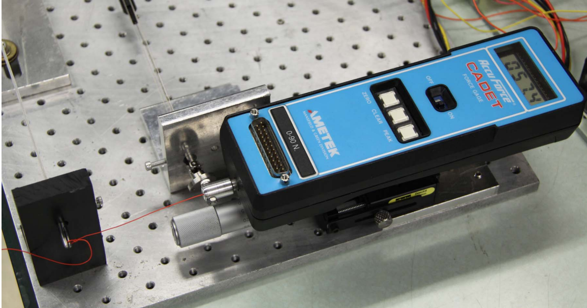
Figure 5.6: Experiment setup of measuring gripping force of gripper
