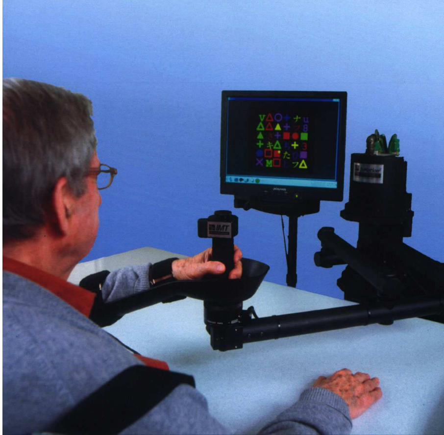
Figure 1.1: The Inmotion 2 Shoulder-Elbow Robot is used in upper extremity physical rehabilitation therapies and only allows 2D shoulder-elbow movements [1].
