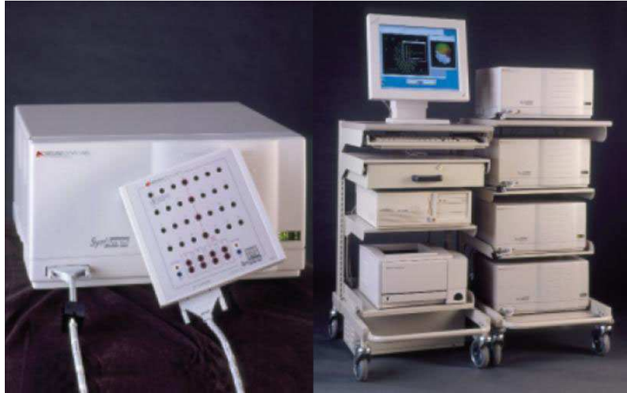
Figure 4.3: Photograph of the NeuroScan Synamps amplifier system used to make EEG recordings in this study [5].
