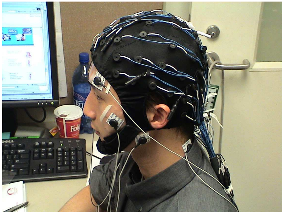
Figure 4.2: Photograph of the NeuroScan 64-electrode Quick-Cap used to make EEG recordings in this study.
