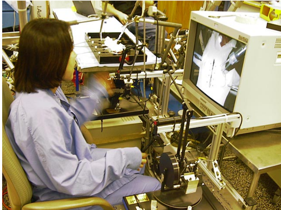
Figure 2.4: Master workstation of the RTW.
