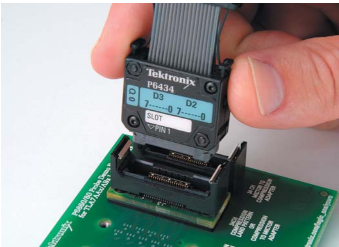
Figure 5. High-density, multi-channel logic analyzer probe.
