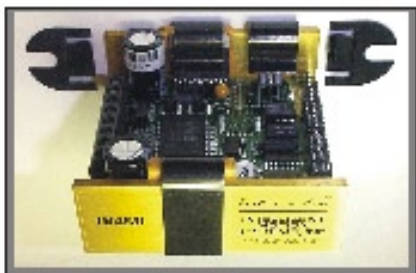
Figure D.2-A: Clips being installed on an IM483
