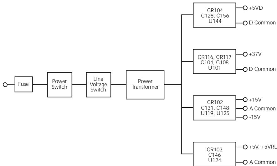
AC power is applied to the AC power module receptacle (J1009). Power is routed through the line fuse and line voltage selection switch of the power module to the power transformer. The power transformer has a total of four secondary windings for the various supplies.
