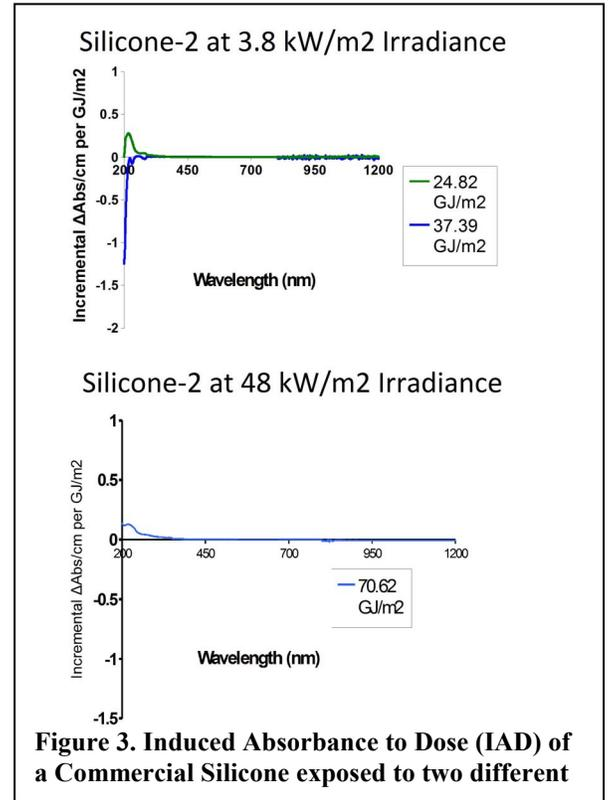
**Figure 3. Induced Absorbance to Dose (IAD) of a Commercial Silicone exposed to two different**
