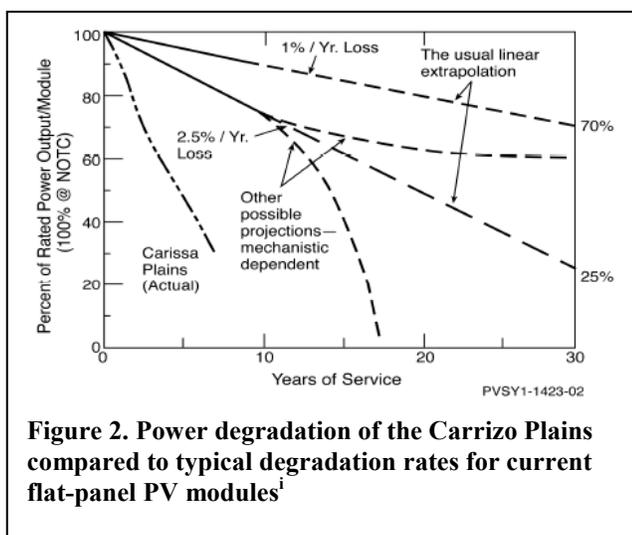
**Figure 2. Power degradation of the Carrizo Plains compared to typical degradation rates for current flat-panel PV modules<sup>i</sup>**
