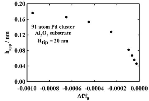
**Figure 4.** The apparent height  $h_{\text{app}}$  of a 91-atom cluster of Pd on  $\text{Al}_2\text{O}_3$  interacting with a 20 nm Si tip shown as a function of the frequency shift setpoint  $\Delta f/f_0$ . Note that the apparent height becomes larger as the setpoint is made more negative. At setpoints more negative than shown here, the feedback becomes unstable, as discussed in the text.
