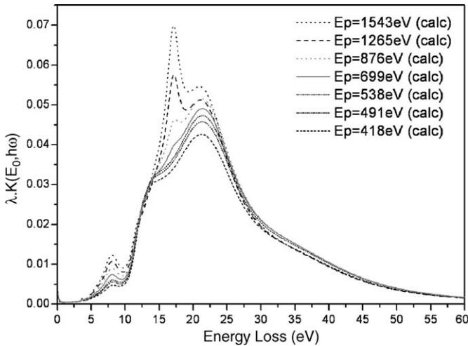
Fig. 12. Comparison of the fitted single scattering cross-sections at different primary energies ranging from  $E_p = 418$  to  $1543$  eV.
