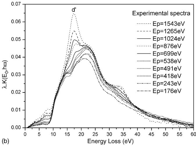
Fig. 3. Single scattering cross-section derived from the experimental REELS spectra of the 2 m SiO<sub>2</sub> layer on Si substrate: (a)  $E_p = 176, 243, 418$  eV; (b) from  $E_p = 176$  to 1543 eV.
