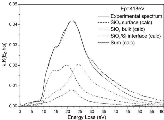
Fig. 13. Decomposition of the experimental scattering cross-sections at  $E_p = 418$  eV into bulk, surface and interface contributions following Eq. (5) using the  $(\omega_j, f_j, \gamma_{j\text{REELS}})$  parameters from Tables 4 and 6.
