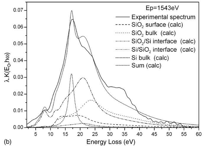
Fig. 11. Decomposition of the experimental single scattering cross-section at  $E_p = 1423$  eV into bulk SiO<sub>2</sub>, surface SiO<sub>2</sub>, interface Si/SiO<sub>2</sub>, and bulk Si contributions. The interface contribution is twofold, see Eq. (5) (coefficients *C* and *D*). The parameters of the dielectric function for Si and SiO<sub>2</sub> are: (a) the ( $\omega_j, f_j, \gamma_j$  optical) values; (b) the ( $\omega_j, f_j, \gamma_j$  REELS) values from Tables 4 and 6.
