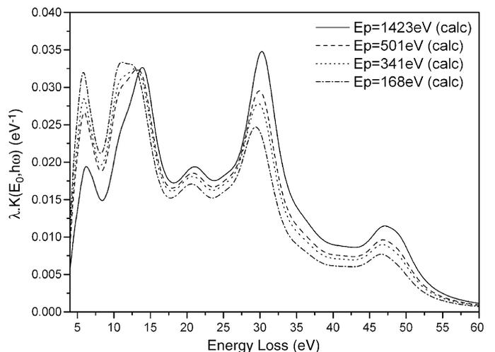
Fig. 8. Comparison of the fitted single scattering cross-sections at  $E_p = 1423$ , 501, 341 and 168 eV. These fitted single scattering cross-sections are labelled “surface + bulk (calc)” in Fig. 7a–d.
