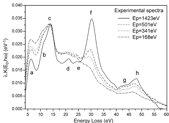
Fig. 2. Single scattering cross-section derived from the experimental REELS spectra of SrTiO<sub>3</sub> ( $E_p = 168, 341, 501$  and 1423 eV).
