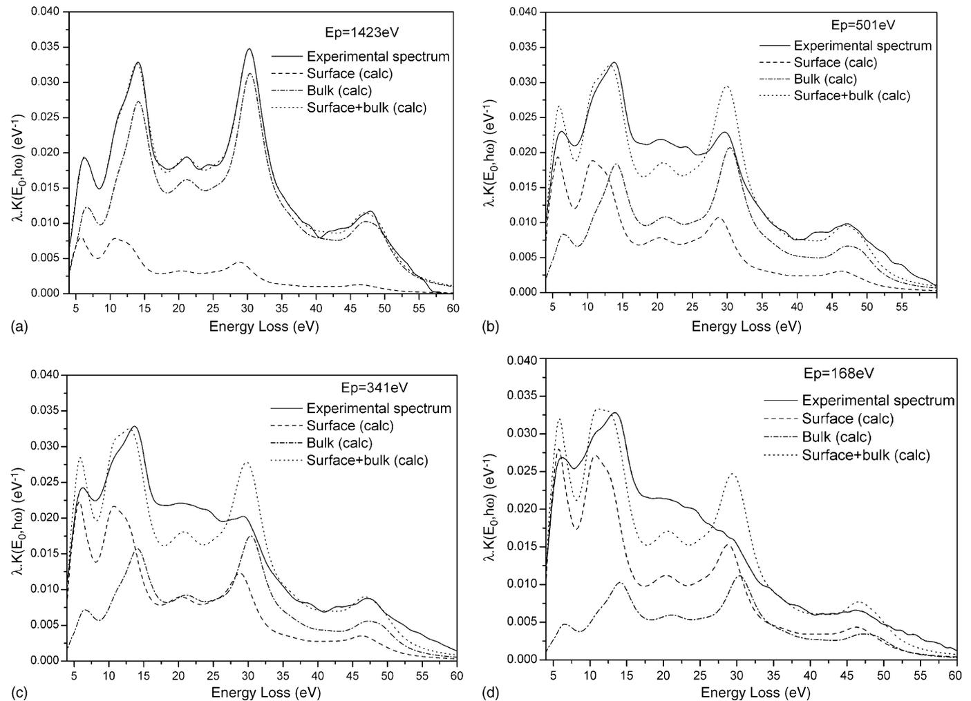
Fig. 7. Decomposition of the experimental single scattering cross-section into bulk and surface contributions, by using the parameters  $(\omega_j, f_j, \gamma_j)_{\text{REELS}}$  from Table 1 for the dielectric function of SrTiO<sub>3</sub>: (a)  $E_p = 1423$  eV; (b)  $E_p = 501$  eV; (c)  $E_p = 341$  eV; (d)  $E_p = 168$  eV.
