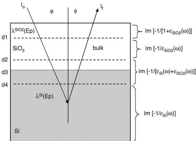
Fig. 5. Si substrate (in grey) covered by a SiO<sub>2</sub> layer (in white). The  $d_1$ – $d_4$  distances are used in Eqs. (6)–(10).
