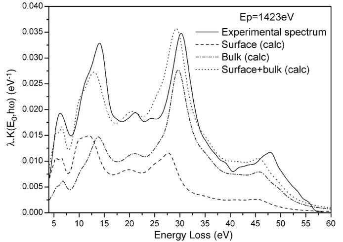
Fig. 6. Decomposition of the experimental single scattering cross-section at  $E_p = 1423$  eV into bulk and surface contributions, by using the parameters  $(\omega_j, f_j, \gamma_j)_{\text{TEELS}}$  from Table 1 for the dielectric function of SrTiO<sub>3</sub>.
