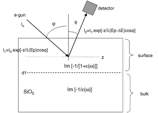
Fig. 4. Geometry of the REELS experiment, in the case of a homogeneous sample with a solid/vacuum interface. The  $d_1$  distance is used in Eqs. (2) and (3).
