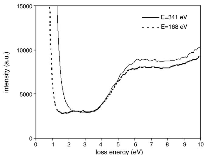
Fig. 1. Low loss energy part of the REELS spectra of SrTiO<sub>3</sub> ( $E_p = 341$  and 168 eV).
