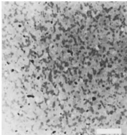
Fig. 5. Backscattered image of Ti(CN)-30% TiB<sub>2</sub> material (bar=10 μm).
