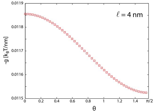
FIG. 5. (Color online) Retarded dispersion interaction between (6,5) SWCNT and a half space made of (6,5) SWCNTs as a function of the angle  $\theta$  between the longitudinal axes of the two subsystems. The distance between the two subsystems is  $\ell=4$  nm.
