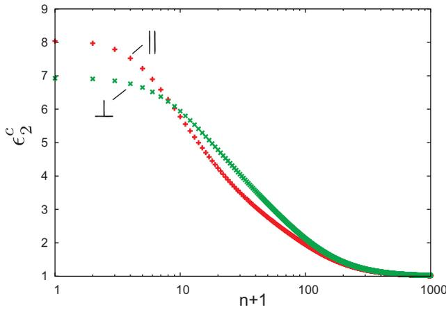
FIG. 4. (Color online) Dielectric responses (along imaginary axis) of the (6,5) SWCNT. The (red) pluses and (green)  $\times$ 's show the longitudinal and transverse responses, respectively. On the  $x$ -axis is the (shifted) Matsubara frequency index.
