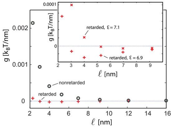
FIG. 7. (Color online) Retarded (crosses) and nonretarded (circles) vdW interactions between a (6,5) CNT and golden half space as a function of distance. The parameters of the medium are  $m=17$ ,  $\sigma=2$ , and  $\mathcal{E}=6.9$ . The inset shows how the retarded vdW interaction depends on  $\mathcal{E}$  for  $\mathcal{E}=6.9$  and  $\mathcal{E}=7.1$ .
