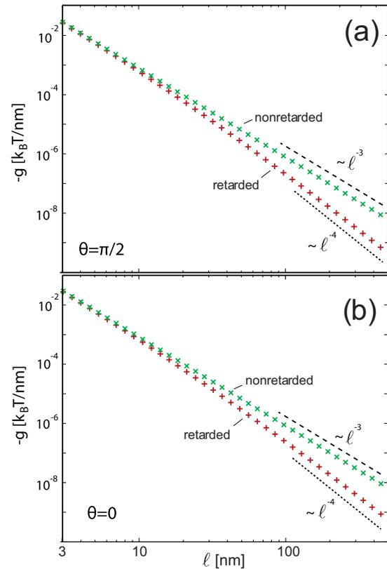
FIG. 3. (Color online) vdW interaction for a (6,5) carbon nanotube above a half space made of (6,5) carbon nanotubes as a function of distance ( $\epsilon_3=1$ ) for  $\theta=\pi/2$  (panel a) and  $\theta=0$  (panel b). The values of dispersion interaction with retardation included are indicated by (red) pluses. The nonretarded values are indicated by (green)  $\times$ 's. The power-law behaviors  $\ell^{-4}$  and  $\ell^{-3}$  are denoted by dotted and dashed lines, respectively.
