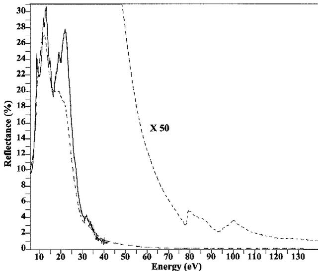
Fig. 8. Comparison of reflectance of  $\alpha\text{-Al}_2\text{O}_3$  between VUV and EELS (dashed line) data after KK analysis.
