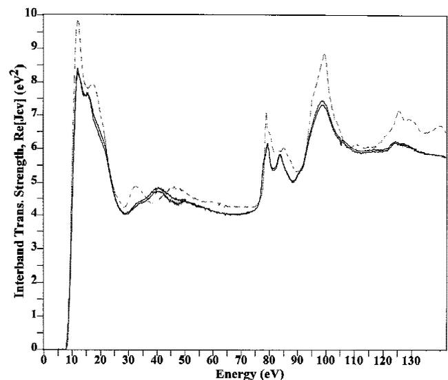
Fig. 11. Interband transition strength,  $\text{Re}(J_{cv})$ , of thin-film  $\gamma$ - and  $\delta\text{-Al}_2\text{O}_3$ , determined by KK analysis of EELS data with results for  $\alpha\text{-Al}_2\text{O}_3$  (dashed line) shown for comparison.
