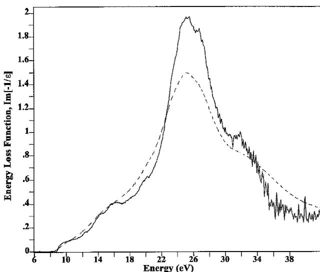
Fig. 9. Comparison of energy-loss functions of  $\alpha\text{-Al}_2\text{O}_3$  determined from KK analysis of VUV and EELS (dashed line) data.
