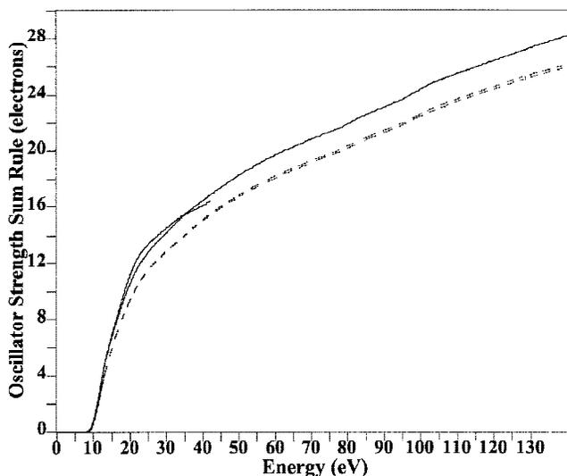
Fig. 13. Oscillator strength sum rules for three phases of  $\text{Al}_2\text{O}_3$ , calculated on an  $\text{Al}_2\text{O}_3$  formula-unit basis. Sum rules for  $\alpha$ - $\text{Al}_2\text{O}_3$  from both VUV and EELS data (solid lines) and thin-film  $\gamma$ - and  $\delta$ - $\text{Al}_2\text{O}_3$  (dashed lines) are shown.
