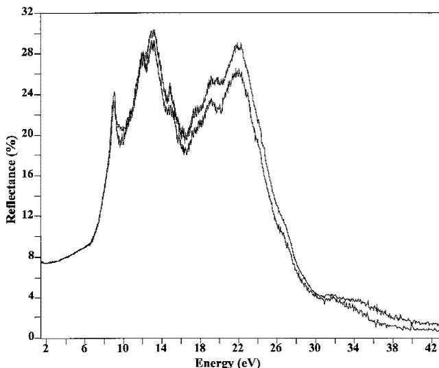
**Fig. 1.** Reflectance of single-crystal α-Al<sub>2</sub>O<sub>3</sub>, for  $E$  perpendicular to  $c$ -axis, determined using VUV and UV/visible spectroscopies.
