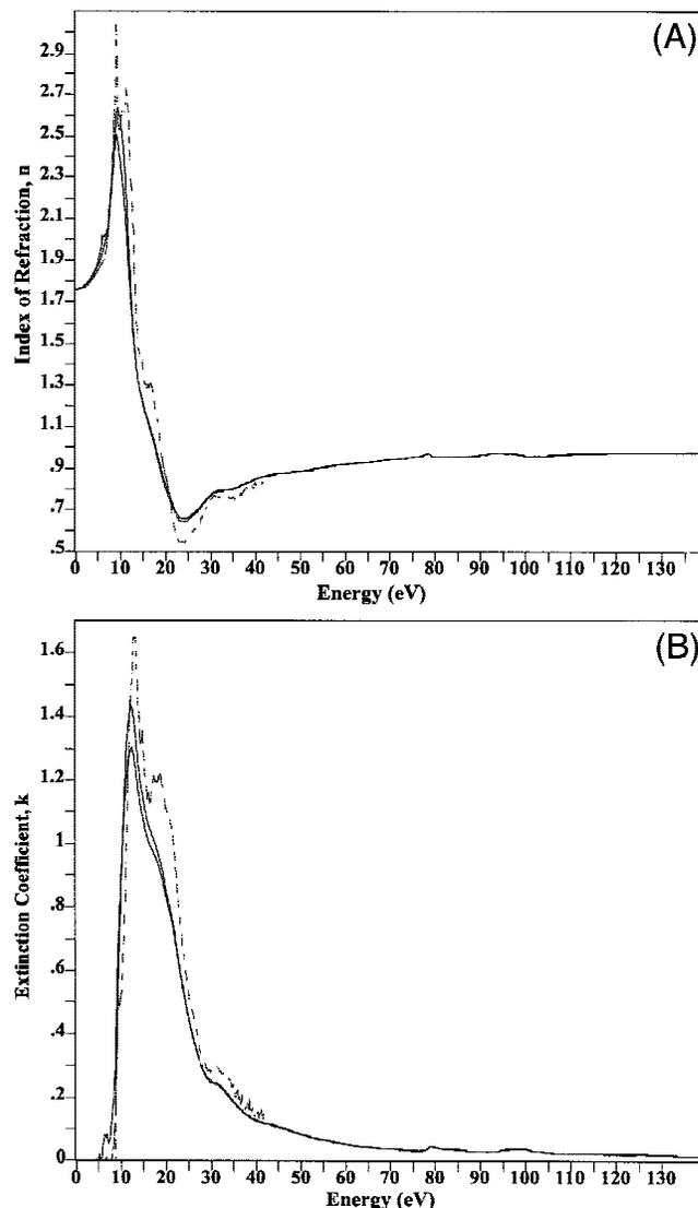
Fig. 7. Complex index of refraction ( $n + ik$ ) consisting of (A) the index of refraction and (B) the extinction coefficient of thin-film  $\alpha\text{-Al}_2\text{O}_3$ , determined by KK analysis of EELS data. Results from KK analysis of VUV data also are shown (dashed lines).
