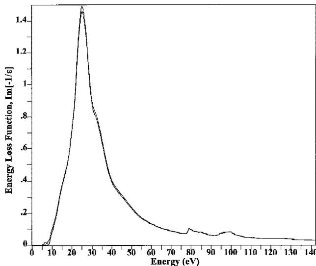
Fig. 5. Energy-loss functions for thin-film  $\alpha\text{-Al}_2\text{O}_3$  after single-scattering correction and zero-loss peak removal.
