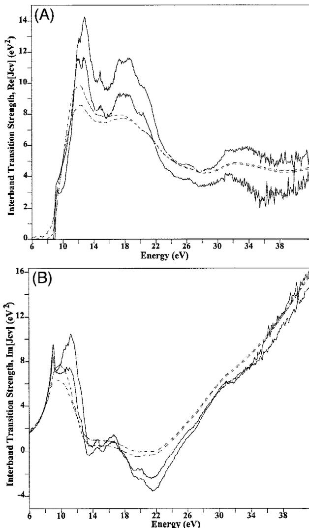
**Fig. 2.** Interband transition strength: (A)  $\text{Re}[J_{cv}]$  and (B)  $\text{Im}[J_{cv}]$  of single-crystal α-Al<sub>2</sub>O<sub>3</sub>, for  $E$  perpendicular to the  $c$ -axis, determined by KK analysis of VUV and UV/visible reflectance data. For comparison, the results from KK analysis of EELS data of α-Al<sub>2</sub>O<sub>3</sub> also are shown (dashed lines).
