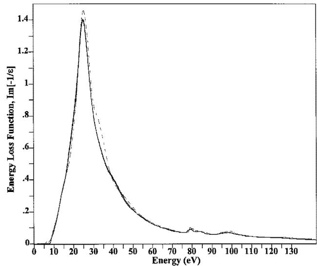
Fig. 10. Energy-loss functions from EELS data for thin-film  $\gamma$ - and  $\delta\text{-Al}_2\text{O}_3$  after single-scattering correction and zero-loss peak removal with results for  $\alpha\text{-Al}_2\text{O}_3$  (dashed line) shown for comparison.
