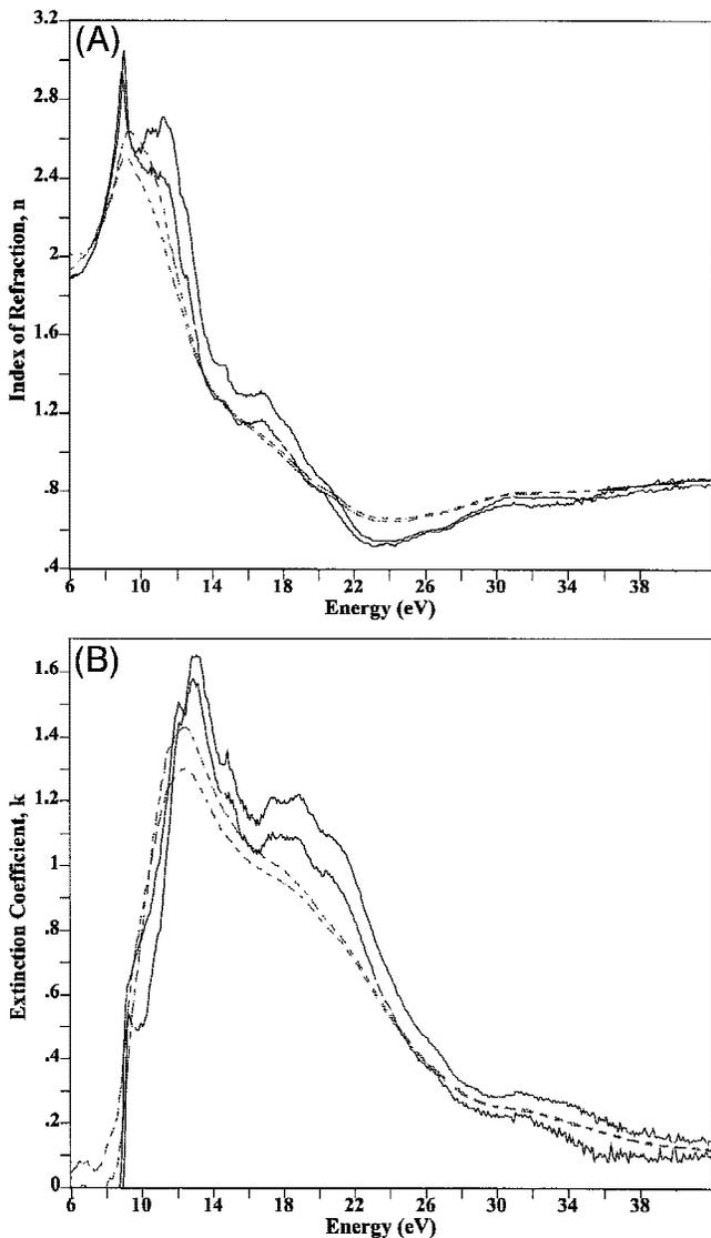
Fig. 3. Complex index of refraction ( $n + ik$ ) consisting of (A) the index of refraction and (B) the extinction coefficient of single-crystal  $\alpha\text{-Al}_2\text{O}_3$ , for  $E$  perpendicular to the  $c$ -axis, determined by KK analysis of VUV and UV/visible reflectance data. For comparison, the results from KK analysis of EELS data of  $\alpha\text{-Al}_2\text{O}_3$  also are shown (dashed lines).
