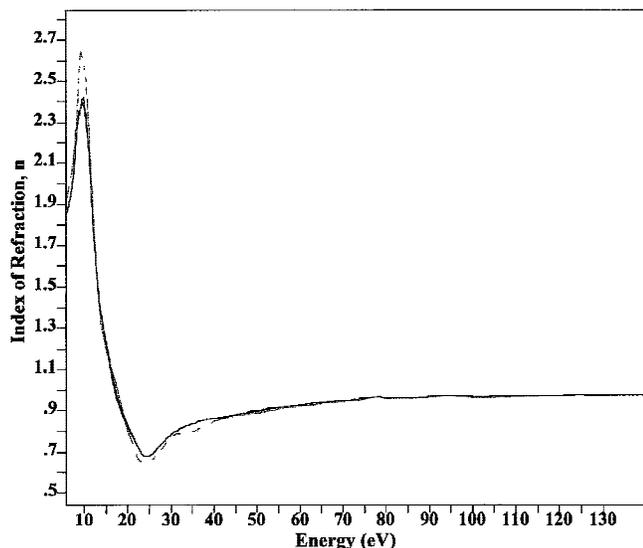
Fig. 12. Index of refraction,  $n$ , of thin-film  $\gamma$ - and  $\delta$ - $\text{Al}_2\text{O}_3$ , determined by KK analysis of EELS data with results for  $\alpha$ - $\text{Al}_2\text{O}_3$  (dashed line) shown for comparison.
