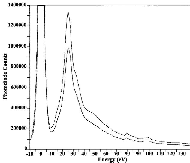
Fig. 4. Raw EELS spectra for thin-film  $\alpha\text{-Al}_2\text{O}_3$  measured using STEM. These spectra show the zero-loss peak (0 eV), the plasmon peak (26 eV), the effects of multiple scattering ( $\sim 50$  eV), and the aluminum  $L$ -edge ( $>78$  eV).
