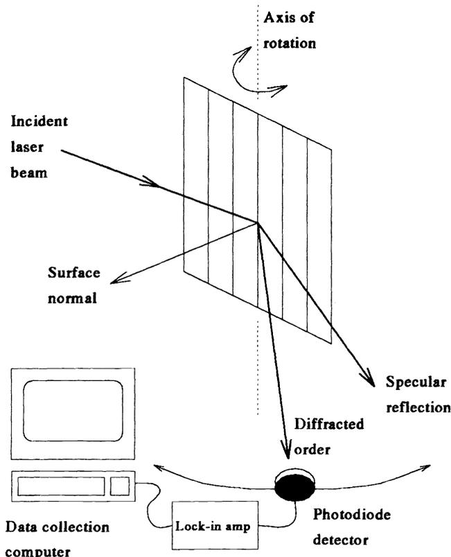
Figure 5. Research grade scatterometer.
