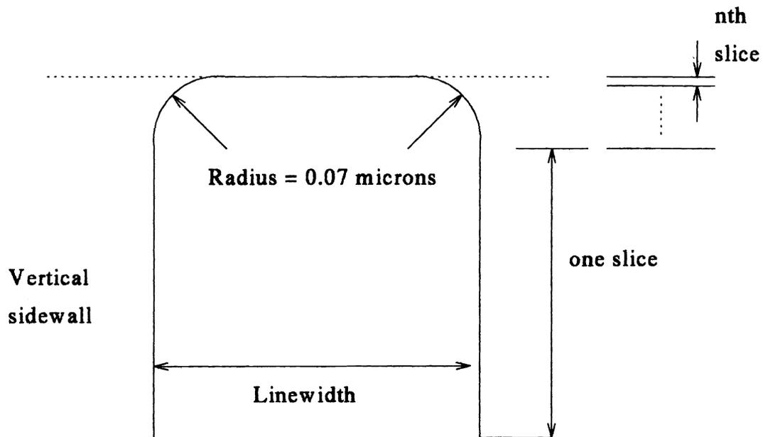
Figure 3. Quartz rounded top corner profile.
