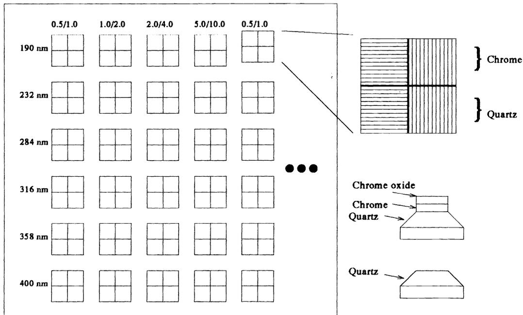
Figure 1. AT&T photomask layout.
