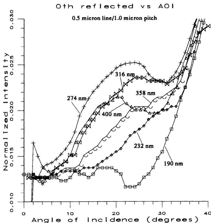
Figure 6. Experimental 0<sup>th</sup> reflected diffracted order for different etch depths.
