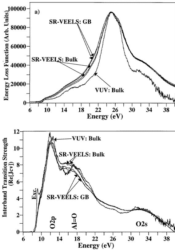
**Figure 2.** (a) Single scattering deconvoluted STEM VEELS spectra for two locations in Grain 1 and 2 and two locations along the near- $\Sigma 11$  tilt grain boundary compared with VUV EELS spectra and (b) the interband transition strength (in  $\text{eV}^2$ ) determined by Kramers Kronig analysis of these VEELS spectra compared with those determined by Kramers Kronig analysis of VUV reflectance spectra.
