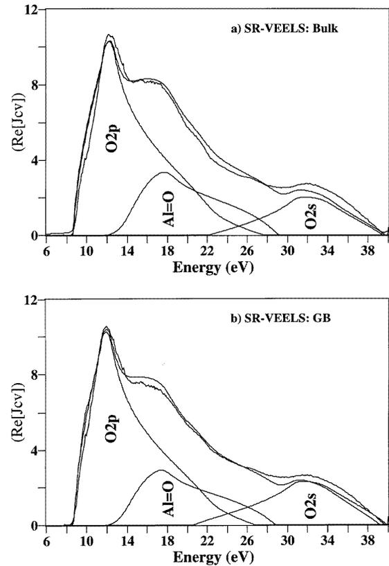
**Figure 4.** Critical point models of the interband transitions from STEM VEELS data of  $\alpha$ -Al<sub>2</sub>O<sub>3</sub>, showing the critical point set corresponding to the interband transitions from the O 2p bands, Al=O hybridized bands and the O 2s lower valence bands to the Al conduction bands. The critical point models are fitted to (a)  $\alpha$ -Al<sub>2</sub>O<sub>3</sub> bulk grain and (b) the  $\alpha$ -Al<sub>2</sub>O<sub>3</sub> near- $\Sigma$ 11 tilt grain boundary.
