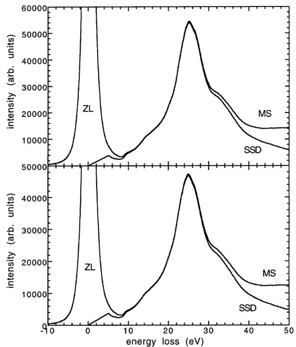
**Figure 1.** Two examples of as-acquired SR VEELS spectra of  $\alpha$ -Al<sub>2</sub>O<sub>3</sub>, with the zero loss (ZL) and multiple scattering (MS) present, and the single scattering deconvoluted (SSD) results obtained using the Gatan routines. Notice the artificial shape where the ZL peak is truncated at 5 eV and also the intensity present below the 8.8 eV band gap even after SSD: the shape of the SSD spectrum determined using these methods is not asymptotic to zero below the band gap.
