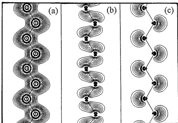
FIG. 3. Distribution of the charge on the Si backbone in Pdn6s. (a) Total valence charge; (b) the HOMO state at  $\Gamma$ ; and (c) the LUMO state at  $\Gamma$ . The contour lines are in the unit of 0.01 to 0.25 by 0.005 electron for (a), and 0.0 to  $0.6 \times 10^{-3}$  by  $0.2 \times 10^{-4}$  electron for (b) and (c).
