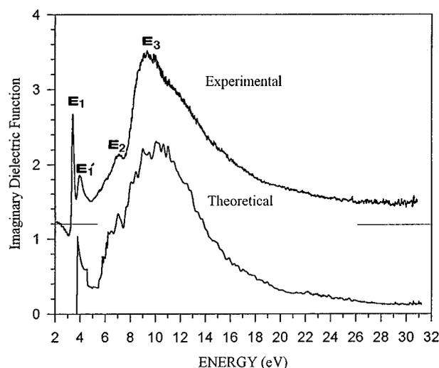
FIG. 5. Comparison of the measured (upper) and calculated (lower)  $\varepsilon_2(\omega)$  curves. The theoretical curve has been compressed towards the lower energy to simulate the effect of an extended basis.
