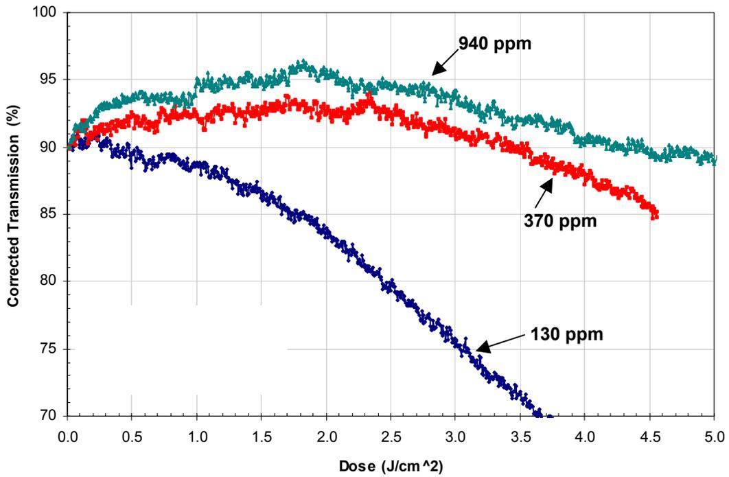
Figure 5: Impact of varying ambient oxygen concentration on pellicle lifetime.
