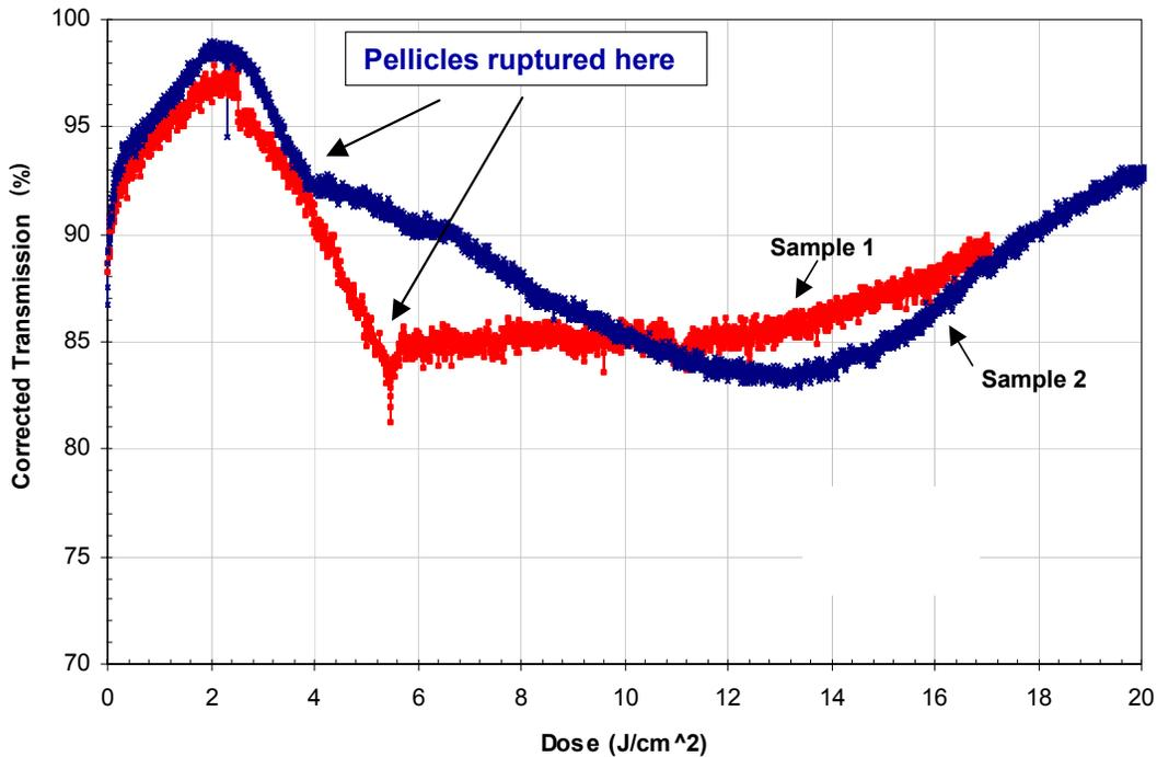
Figure 7: Pellicle laser durability at a high oxygen concentration (1000 ppm).
