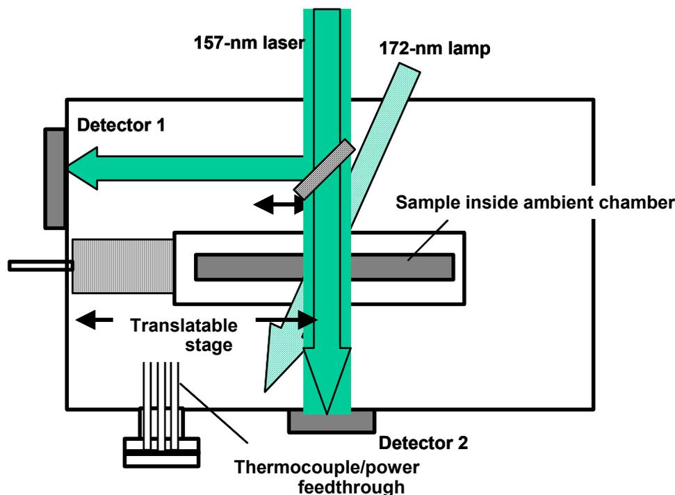
Figure 2: Schematic of pellicle laser irradiation chamber.
