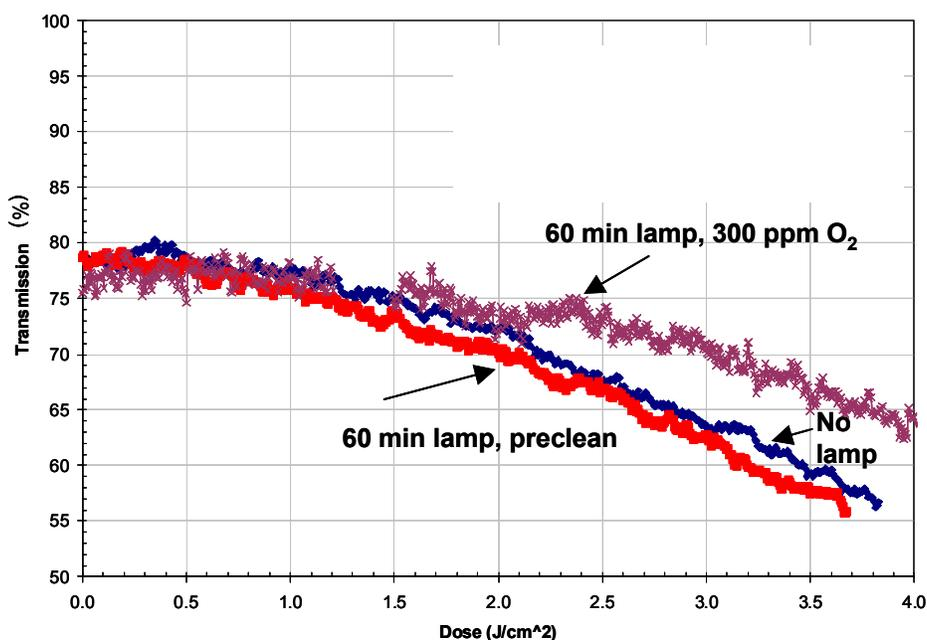
Figure 8: Effect of 172-nm lamp pre-cleaning.
