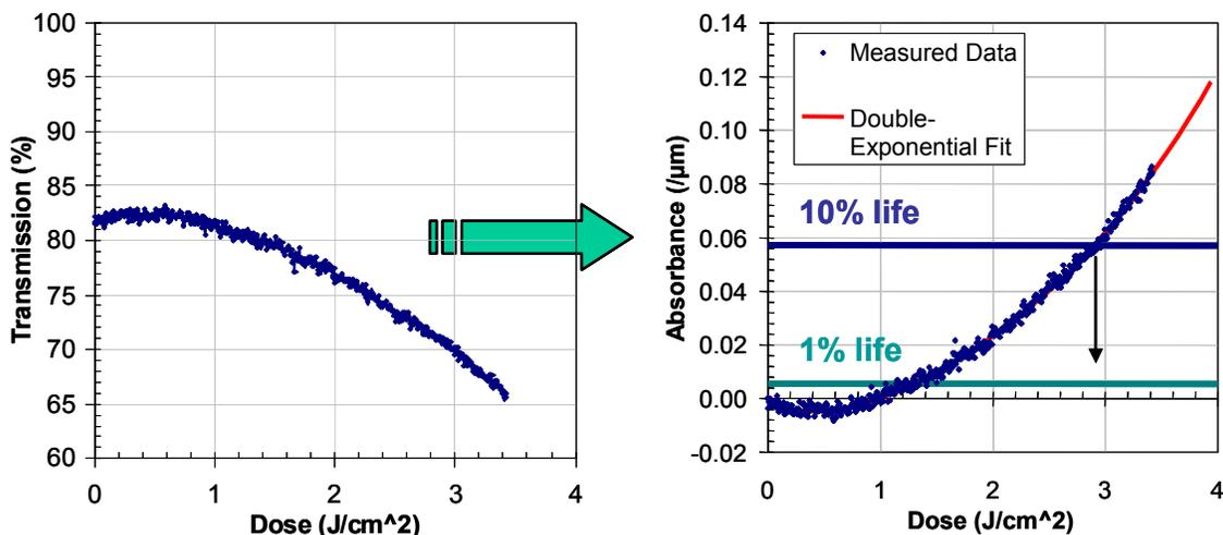
Figure 3: Example of pellicle laser irradiation data. Induced absorbance was calculated from insitu transmission. Lifetime can be read directly from this chart.
