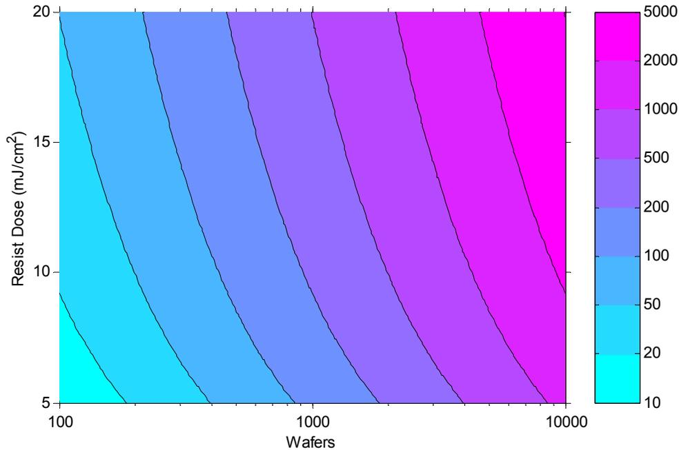
Figure 1: Contour plot illustrating total dose delivered to pellicle (in  $\text{J}/\text{cm}^2$ ) as a function of 300-mm wafers processed and resist dose.
