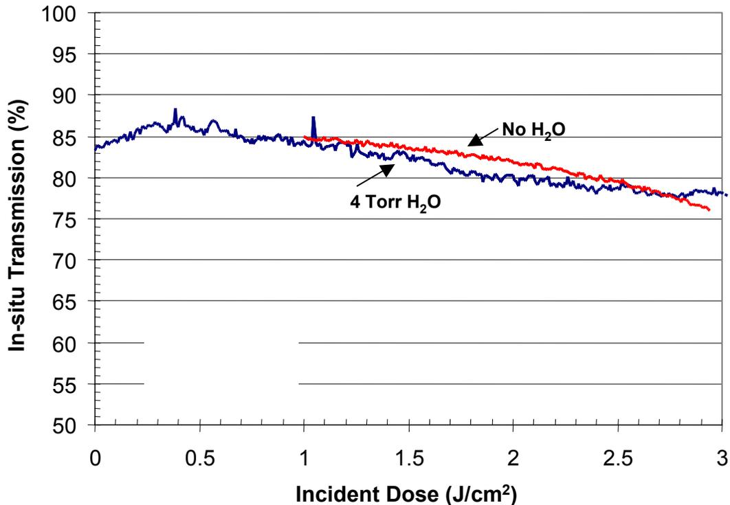
Figure 9: Comparison of pellicle laser durability in high versus low moisture content ambients.
