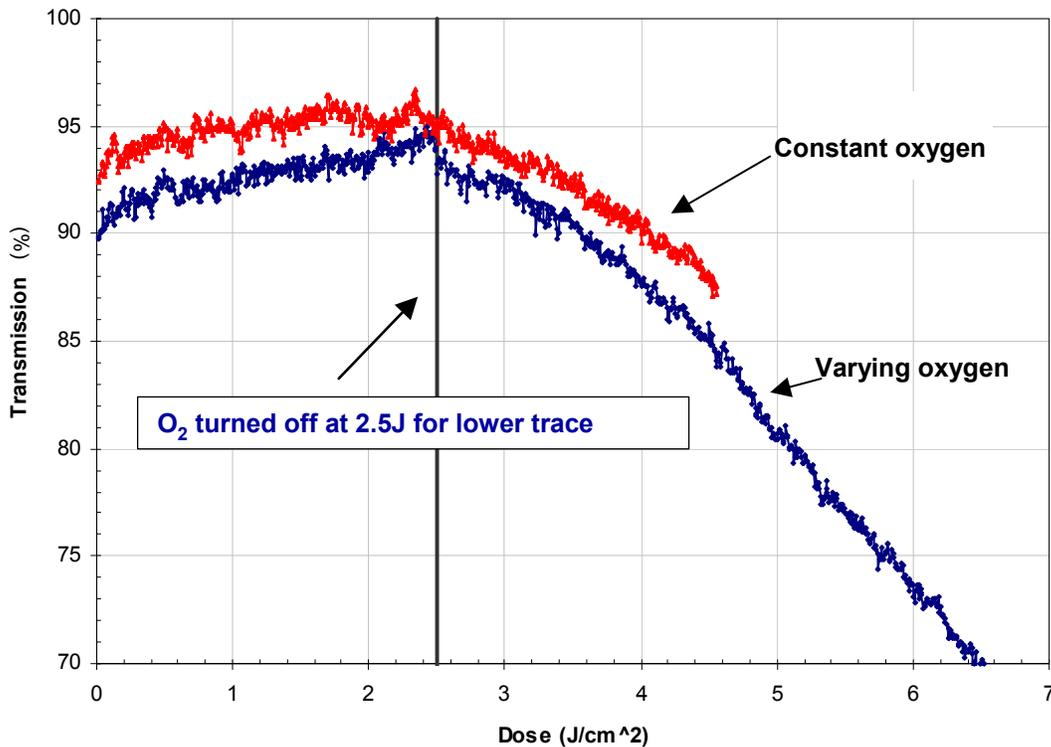
Figure 6: Impact of varying oxygen concentration over time on pellicle lifetime.
