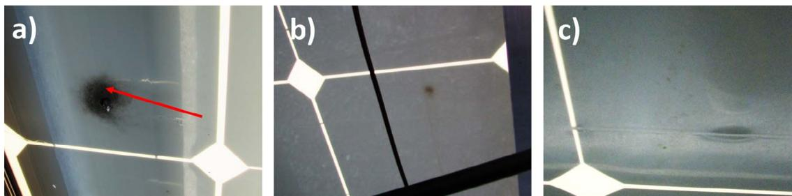
Fig. 2. The two main types of backsheet damage or defects visually observed, including high (a) and low (b) temperature burn-marks, and busbar bumps (c). The arrow in (a) indicates the direction of a scrape.
