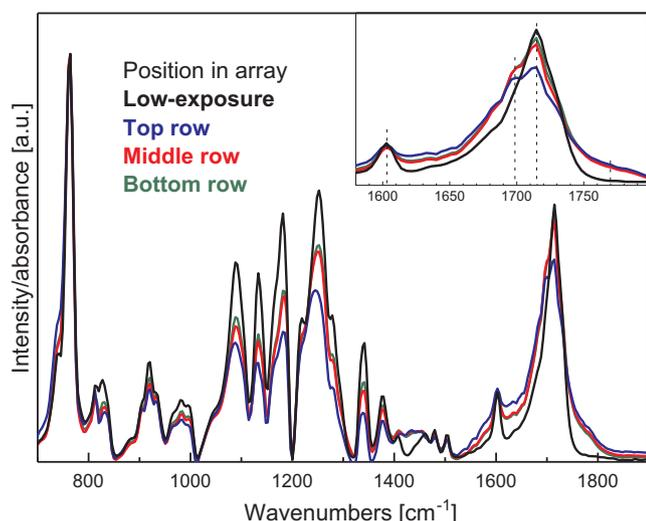
Fig. 4. FTIR spectra from top, middle, and bottom row modules from the center of the sheds. Also shown is a spectrum of a low-exposure PEN backsheet. Inset shows the carbonyl region ( $\approx 1700 \text{ cm}^{-1}$ ). Refer to the online color version for the legend.
