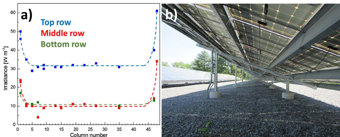
Fig. 5. Backside irradiance around noon on 28 April 2017 at various positions in the array (a). Dashed lines show the trend for each row. A photograph beneath on shed of modules to aid visualization of the backside lighting conditions (b), taken facing east from shed 3-middle row-column 5. Refer to the online color version for the legend.
