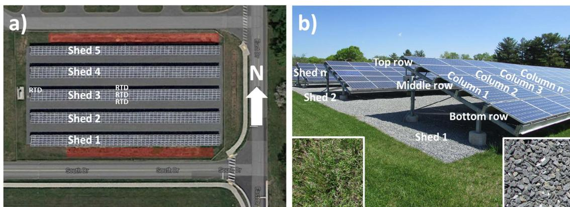
**Fig. 1.** Layout of the NIST ground-mounted PV array (Google Maps, 2016) (a), and orientation of the modules within the array, including nomenclature labels utilized in this work (shed-row-column) (b). “RTD” in (a) marks the approximate location of modules where backside temperature was recorded, and red boxes show the locations of the bio-retention areas (refer to the online color version). Insets for (b) show the ground cover at the array, including grass and coarse rock.
