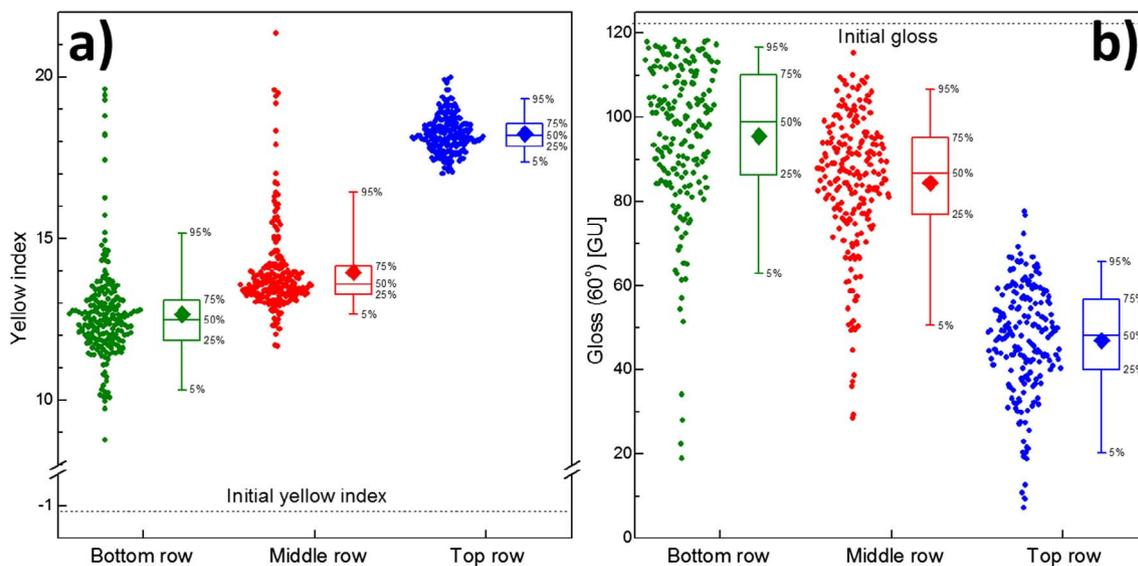
Fig. 3. Yellow index (a) and gloss (60°) (b) for bottom, middle, and top row modules, including mean, median, and various percentile ranges (5%, 25%, 75%, and 95%). Each point represents a single measurement, and there are three measurements per module.
