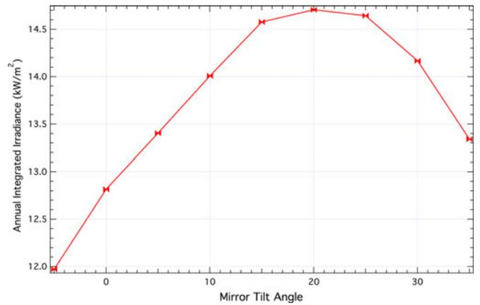
Fig. 7. Plot of the integrated results of Fig 5, showing the total annual irradiance as a function of mirror tilt for a module at 55°. The optimum mirror tilt angle for maximum annual production is 20°, even considering the significant “gullwing” shape of the time-dependent curve, as shown in Fig 5.
