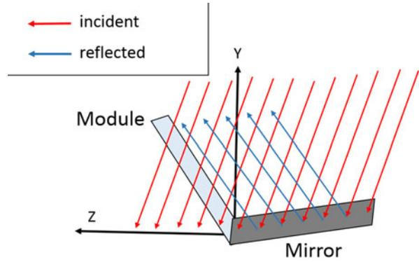
Fig. 6. Explanation of the gullwing shape is provided by TracePro simulation is shown here. Specular reflection rays from the mirror during the summer months of high solar elevation angle do not intercept the PV module at all. This sketch of a TracePro model is taken from June 15 and shows a small subset of incident light rays in red and reflected rays in blue.
