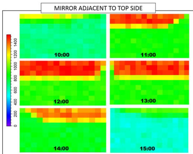
Fig. 3. Irradiance maps across the length and width of a 60-cell Si module, as determined by TracePro. The maps depict the augmentation strength and uniformity near noon time on an hourly basis. It was observed that the nonuniformity created intensity bands across the module length. The mirror adjoins the module at the top of the images.
