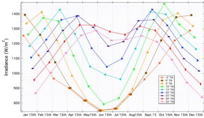
Fig. 5. Simulated peak irradiance upon a module on the 15th day of each month across a calendar year as a function of mirror tilt. The module tilt angle was fixed at 55°, where the optimum value was determined by the 1-D modeling. The curves indicate a “gullwing” shape, where the irradiance is minimum during the summer months.
