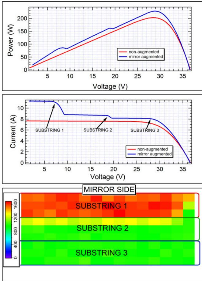
Fig. 8. Comparisons between MAPV and non-MAPV from ray-trace result and field-test site.
