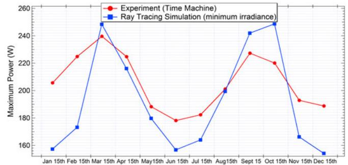
Fig. 9. Time machine measurements of maximum power point of a 200-W 60-cell pc-Si module confirms the gullwing shape of the simulation output for a module at  $55^\circ$  and mirror at  $0^\circ$ .
