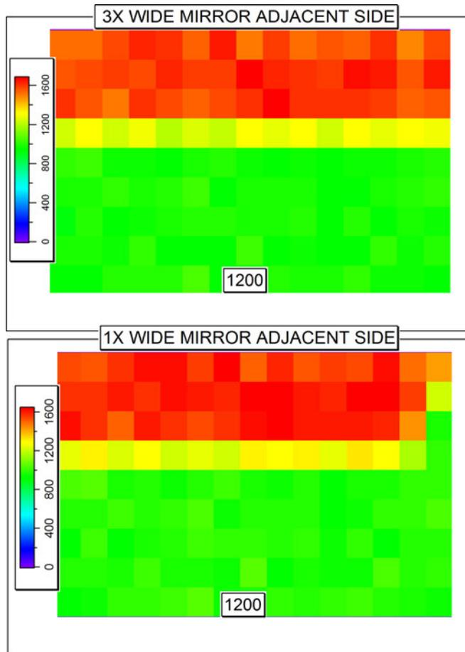
Fig. 4. Edge effects in the irradiance uniformity distribution are eliminated with a mirror that is  $3\times$  longer than the module. This proof-of-concept model was not constructed but suggests that the MAPV modules at the ends of the row should be coupled with mirrors that protrude from the length of the module.
