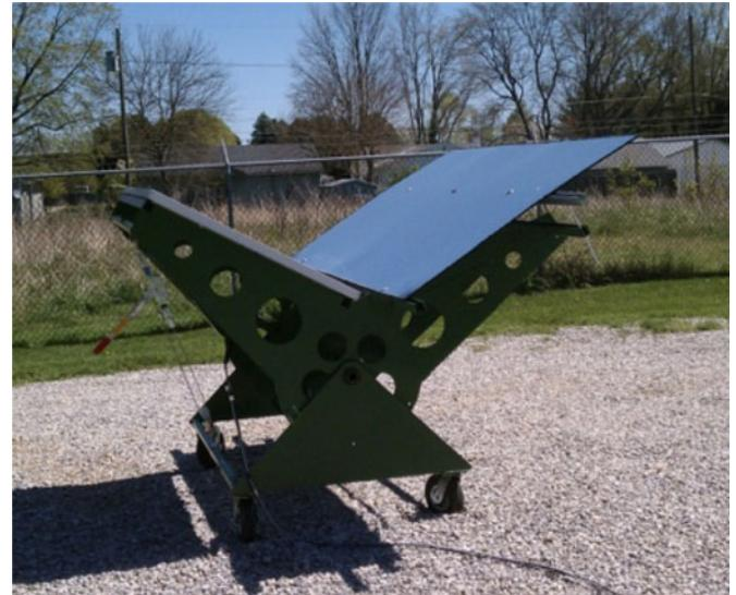
Fig. 2. Replex ‘time machine’: A rotating tilt module/mirror combination that simulates different times of the year by varying the incident angle of the solar irradiance.
