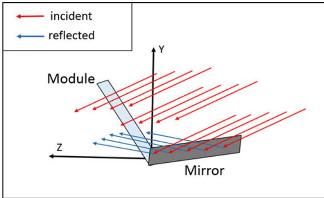
Fig. 1. Sketch of a TracePro 3-D model of a module and mirror system on January 15, with a small subset of the incident solar rays in red and reflected rays in blue.
