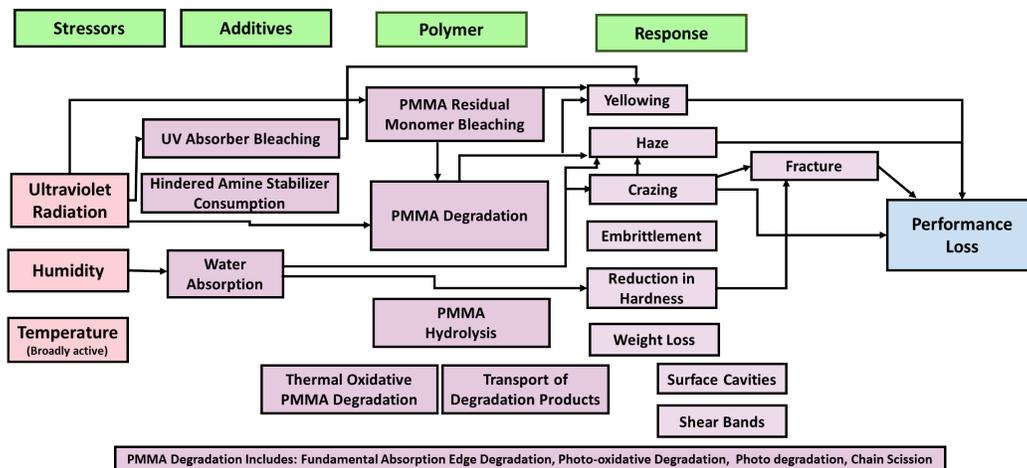
Figure 1. Example Acrylic Degradation Pathway informed by domain analytic shows a sampling of degradation pathways for acrylic based from different stressors.
