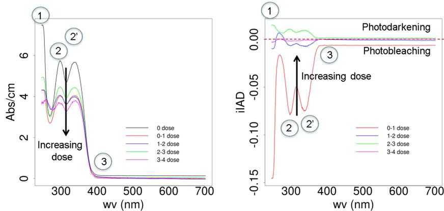
Figure 3. Abs/cm for multipurpose absorbing (MPA) grade poly(methyl methacrylate) (PMMA) for exposures in the QUV accelerated weathering tester to UVA-340 irradiance (irradiance only QUV exposure) for baseline, one to four dose for 1 example samples (left). The corresponding incremental IAD for MPA grade acrylic (right).
