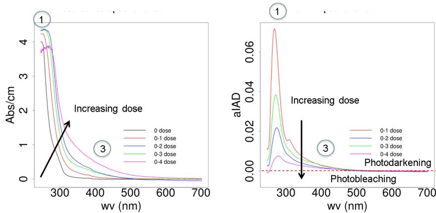
Figure 2. Abs/cm for ultraviolet transparent (UVT) grade poly(methyl methacrylate) (PMMA) for exposures in the QUV accelerated weathering tester to UVA-340 irradiance (irradiance only QUV exposure) for baseline, one to four dose for 1 example samples (left). The corresponding average IAD for UVT grade acrylic (right).
