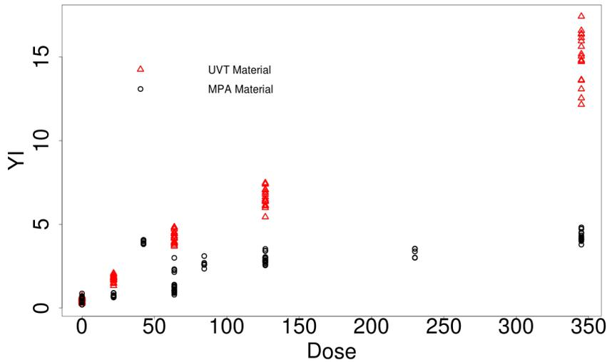
Figure 4. YI values for UVT (triangle) and MPA (circle) grade acrylics for baseline, and one to four dose for all samples.
